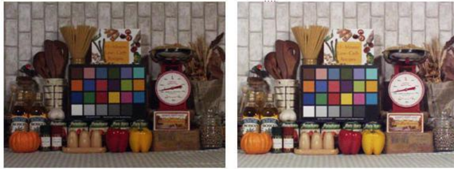
Fig.12 Two sample pictures taken with a front-illuminated camera structure (left) compared to back-illuminated camera structure (right). Sample images taken under low light conditions (30 lux).The CRA related problem (background not uniform) does not exist anymore.
